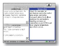
Guided test procedures include connector locations, component operations, meter presets, common faults and expected values.
