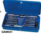
**GA541 U.S. Set** (Blue-Point). Taps and dies from #4 to 1/2" in both NF and NC threads, a pipe thread tap and die, plus 2 die stocks and 3 tap wrenches, a screw pitch gauge and a screwdriver (41 pc) in a storage case.
