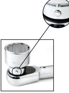
Socket-Lok® button positively locks the socket and drive tool together, providing positive retention and quick disassembly.
