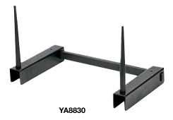
YA8830 Cylinder Head Stand. Holds cylinder head up and away from the workbench, allowing clearance for the manifolds. Steel bar clamps to a bench vise. Simply slide on the movable arms, which adjust to almost any steel or aluminum head configuration.
