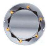
Conventional 12-point wrench and the contact it makes on the corner of a nut or bolt. The corner can round off under high loads causing the wrench to slip.
