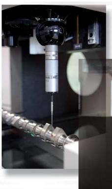
Both the scanning probe and the touch-trigger probe can be optionally equipped with the motorised, rotating/pivoting probe head PH10. Thanks to 3D continuous path control, even inclined holes can be easily measured.
