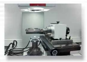
A laterally displaced lifting column in tandem with an SK50 manual swivelling axis allow measurement of tools with large diameters. A glass stage with an SK50 tool holder, is, of course also optionally included in the scope of delivery.
